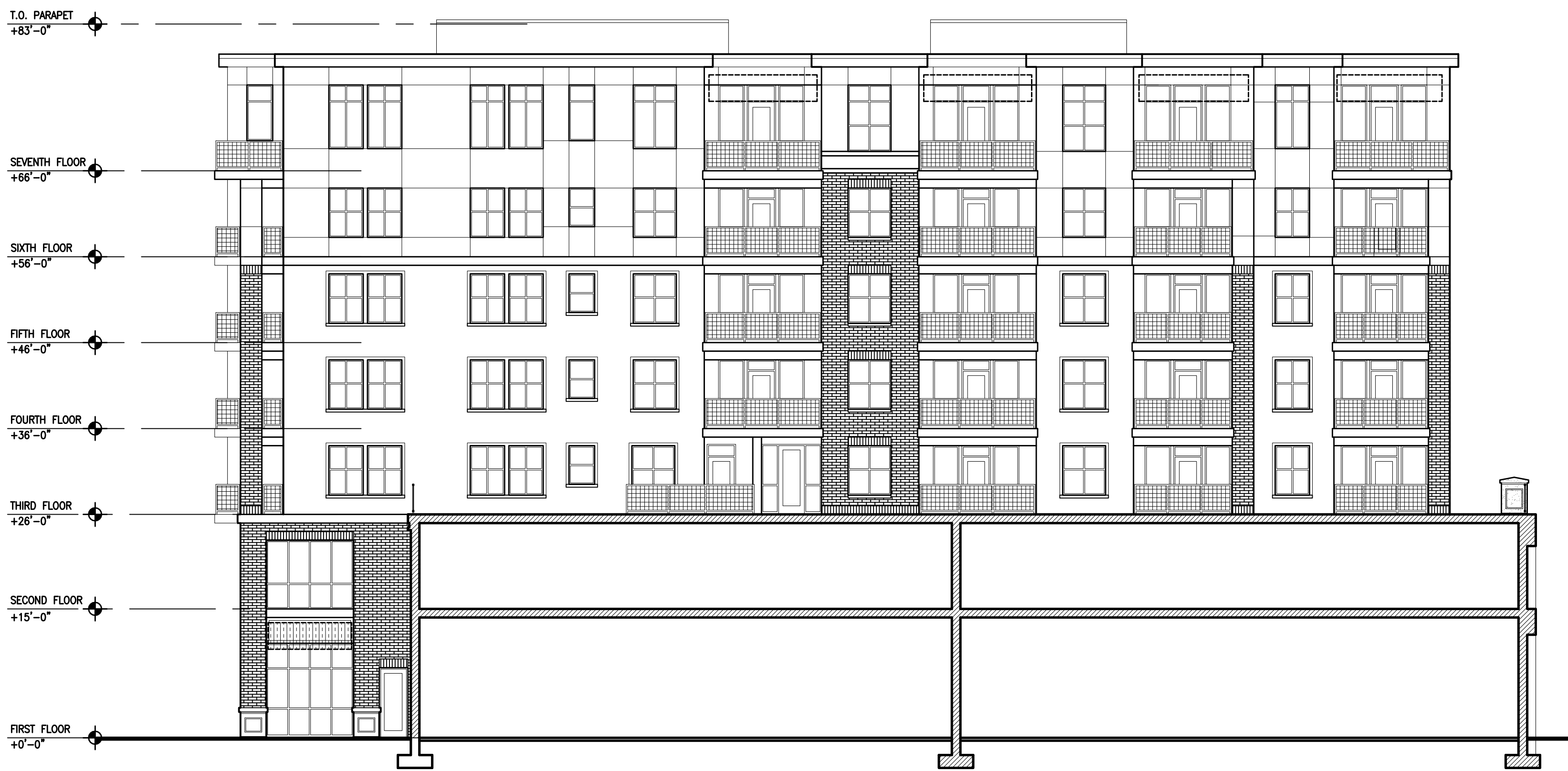
2 BUILDING "B" EAST ELEVATION SCALE: 3/32" = 1'-0"
