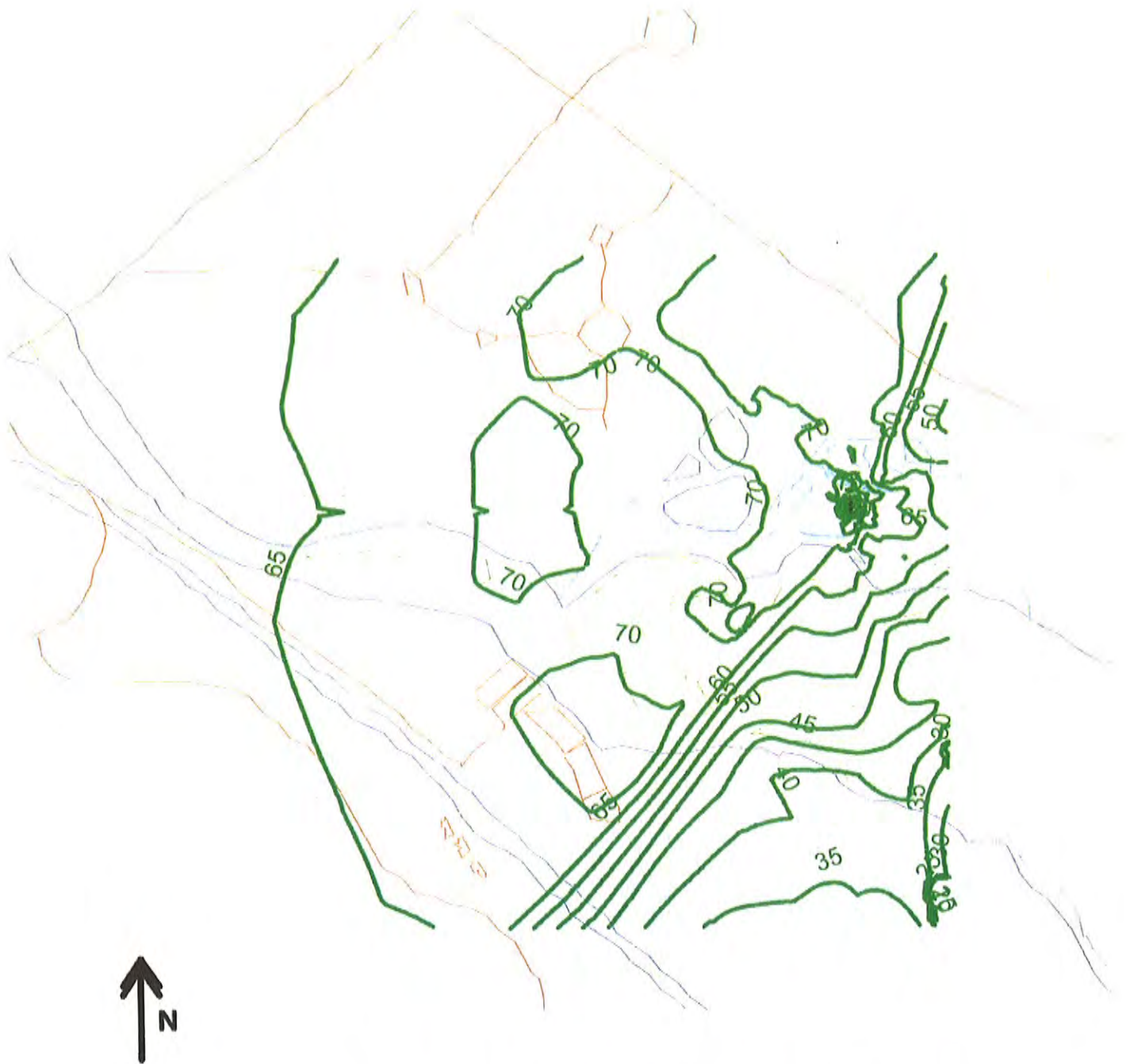
FIGURE 9 PROJECTED NOISE CONTOURS - ORIGINAL CONFIGURATION 60 DEG, 30% HUMIDITY, 3.5 MPH NE WIND, STRONG INVERSION
