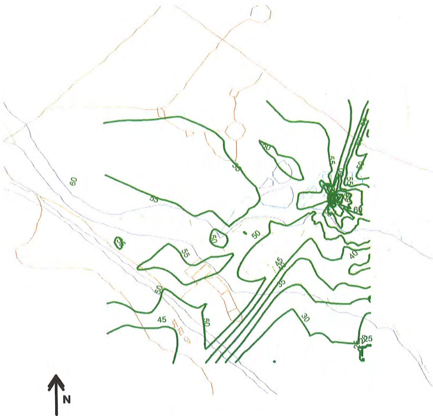
FIGURE 13 PROJECTED NOISE CONTOURS - MOD 4 WITH LIGHT WIND (FROM NE) AND INVERSION
