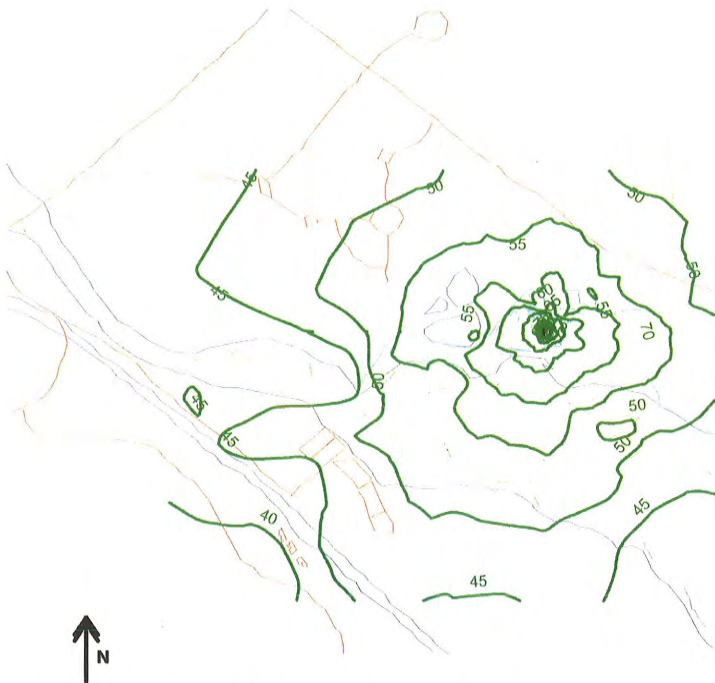
FIGURE 10 PROJECTED NOISE CONTOURS - MOD 1 CONFIGURATION 80 DEG, 80% HUMIDITY, NO WIND, ZERO DEGREE TEMP. GRADIENT
