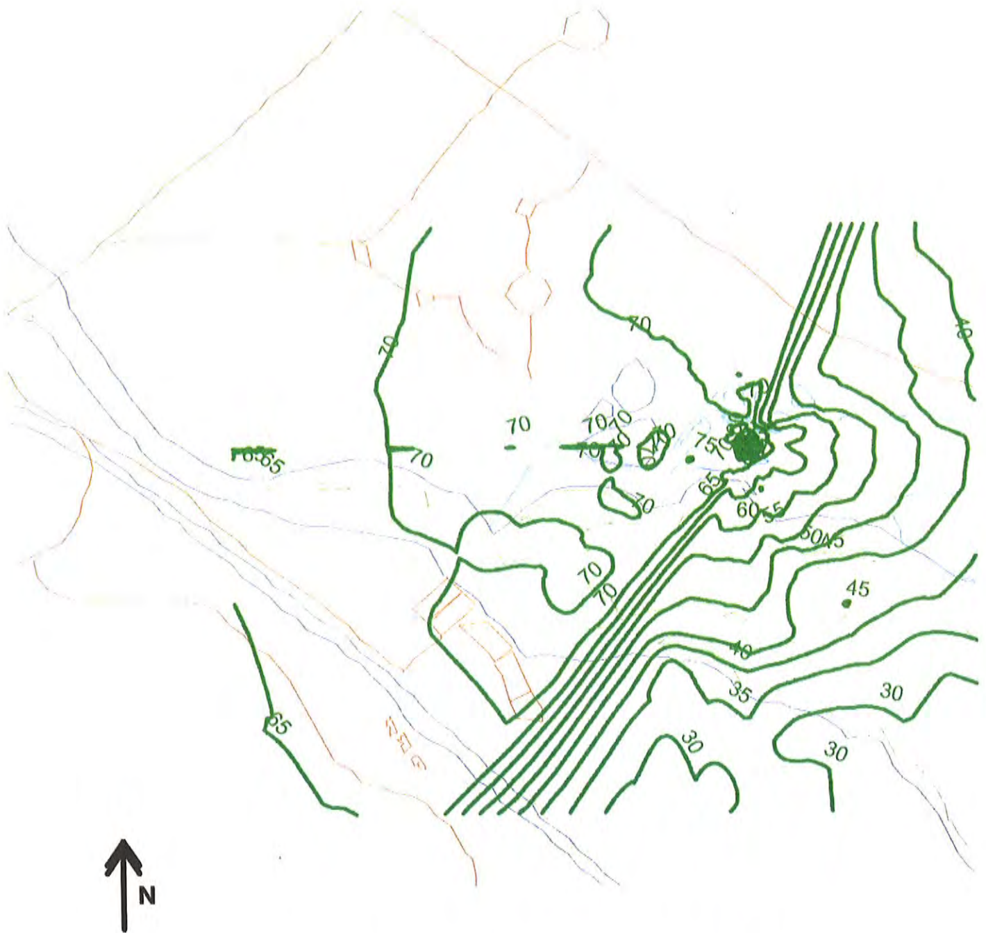
FIGURE 11 PROJECTED NOISE CONTOURS - MOD 1 CONFIGURATION 60 DEG, 30% HUMIDITY, 3.5 MPH NE WIND, STRONG INVERSION
