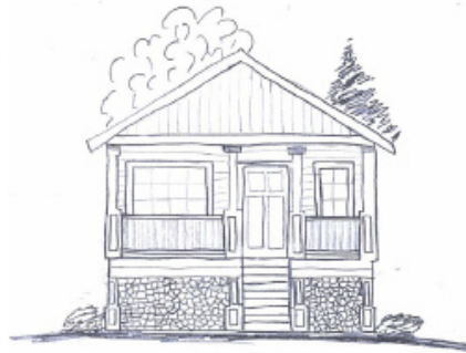
Figure 11-06.6: One and one-half story building
