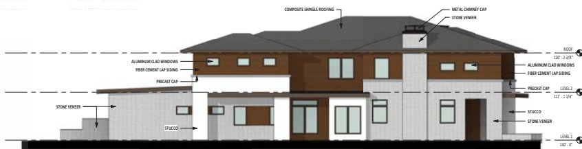
STUDY ELEVATION-UNIT 3A, NORTH 3 CPT2.03A 1/8" = 1'-0"
