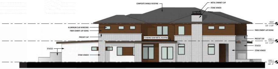
STUDY ELEVATION-UNIT 2A NORTH 3 | CPT2.02A | 1/8" = 1'-0"
