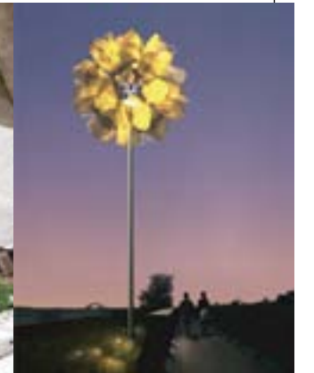
Wind-Powered LED Flower Light, Halton, United Kingdom. As wind blows at speeds above 5 miles an hour, three wind turbines attached to the flower's stem collect energy and power LEDs beneath the petals.
