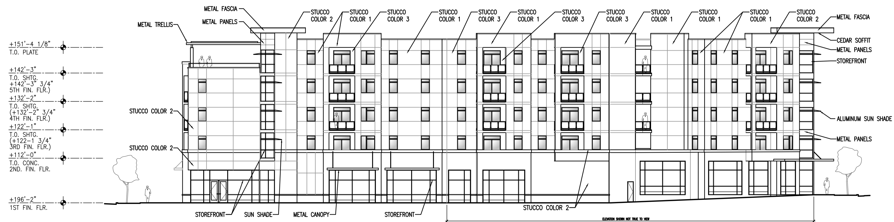
3 NORTH EXTERIOR ELEVATION (W. BEACON AVE.) SCALE: 1/16" = 1'-0"
